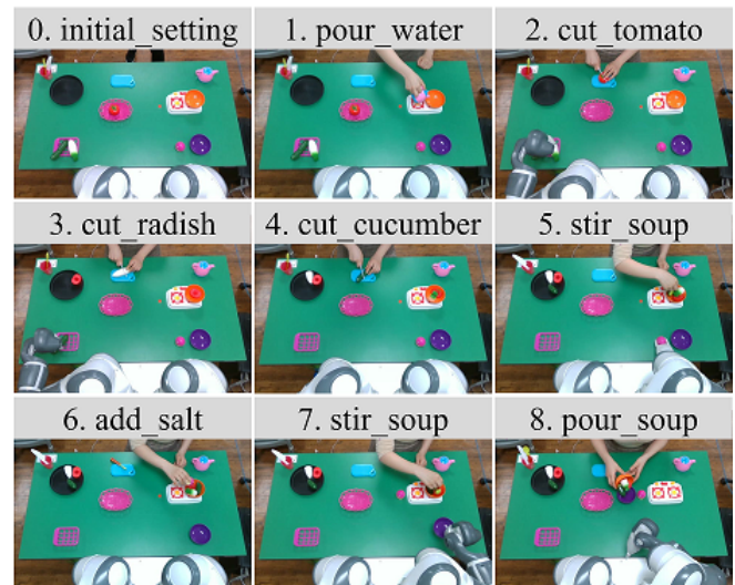
Fig. 1. Brief overview of the main robot system. The robot picks up and hands over objects based on the recognized action and the knowledge about the activity (in the photo 2, 3, 5, and 7)
